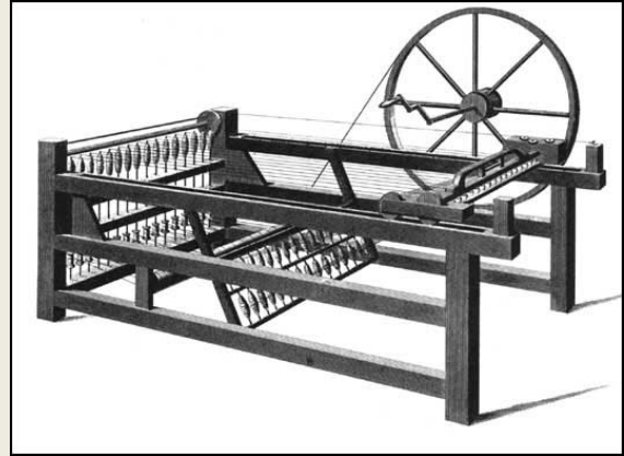
An engraving of a Spinning Jenny by T. E. Nicholson (1835)
