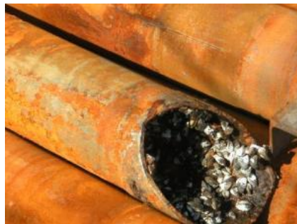
At Lake Ontario in Canada, zebra mussels cling to the inside of a rusty pipe
